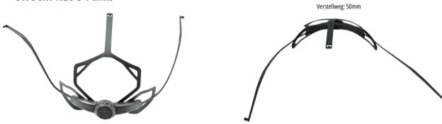
The 3-point version is clicked into the side of the helmet at two attachment points. A ratchet strap on the head spider, connected to an anchor in the EPS, enables individual height adjustment so that the head spider can be optimally adapted to the shape of the head.
